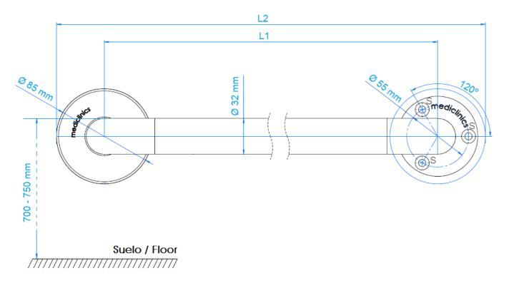
It is not recommended to install the Mediepoxy line bars in places where the bars will be in direct contact with water, in damp and/or chlorinated environments.
